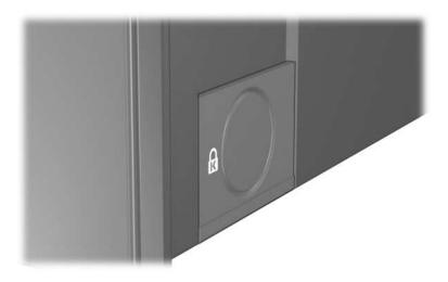
Identifying the Cable Lock Slot
